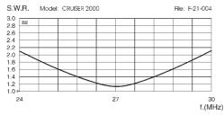
**NOTE:** we recommend following cable's length from transceiver to antenna: 4m, 5m, 7m, 9m, 14m.
