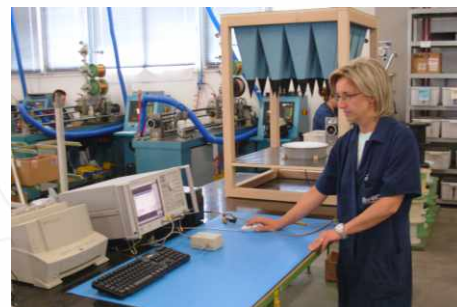
Final test with network analyzer
