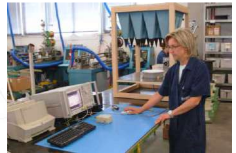
Final test with network analyzer
